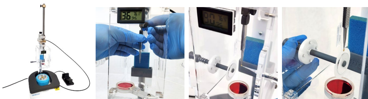
Figure 1. Workflow for sample preparation using the manual plunge cooler. (A) The complete manual plunger assembly. (B) Securing the tweezers (holding the EM grid) to the plunger. (C) Dispensing the sample onto the grid. (D) Blotting the grid to remove excess liquid prior to plunging.
