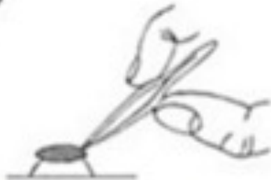
Place the grid on the drop (1 minute)
