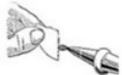
Drain on filter paper
