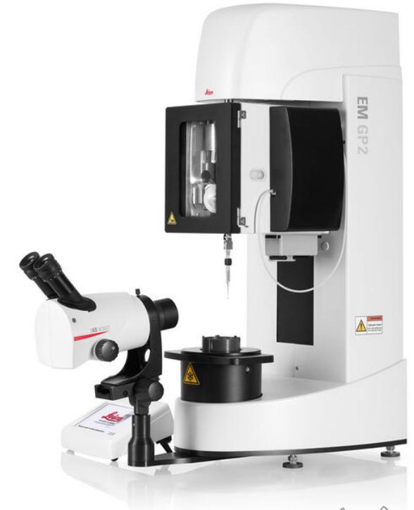
**Examples of guillotine freezing devices**
